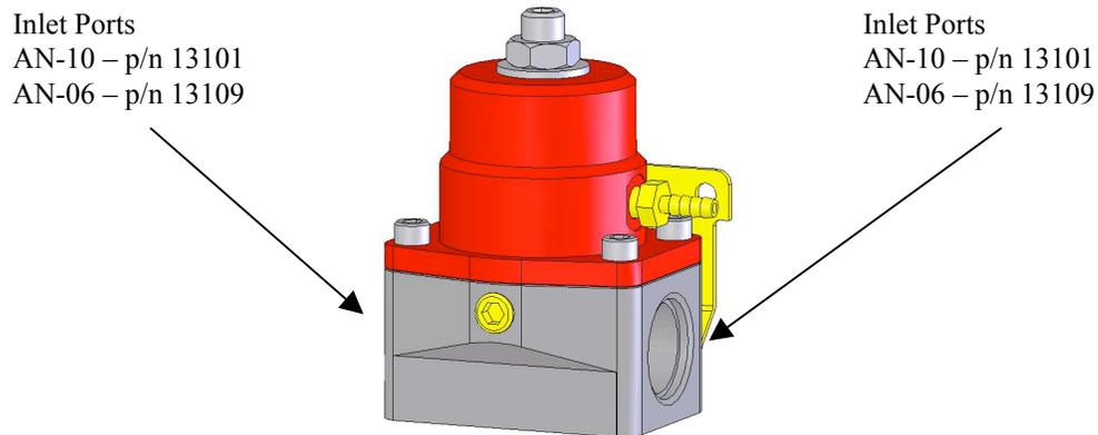
8. Attach the fuel return line to the regulator **bottom** port using an AN-6 style fitting and o-ring.
